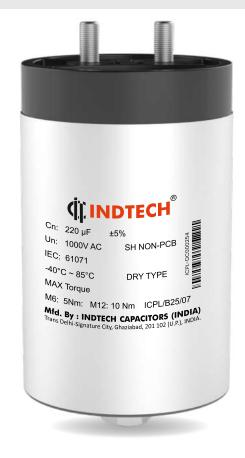
**IGBT snubber capacitors** are essential components in high-power electronic circuits, particularly where Insulated Gate Bipolar Transistors (IGBTs) are employed. These capacitors are designed to mitigate voltage spikes and surges caused by parasitic inductance during switching operations. By providing an alternative path for current flow during rapid transitions, they protect IGBTs from potential damage, thereby enhancing the reliability and performance of the overall circuit.
